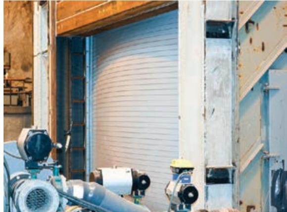
The SafeSpace 500 was subjected to both a positive and negative pressures equal to 1.2 times the 255 mph design wind load.
