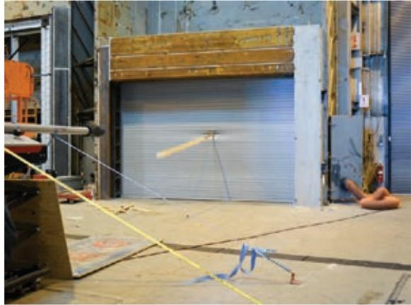
The missile impact test proves the ability to withstand wind-borne debris from a hurricane or tornado.
