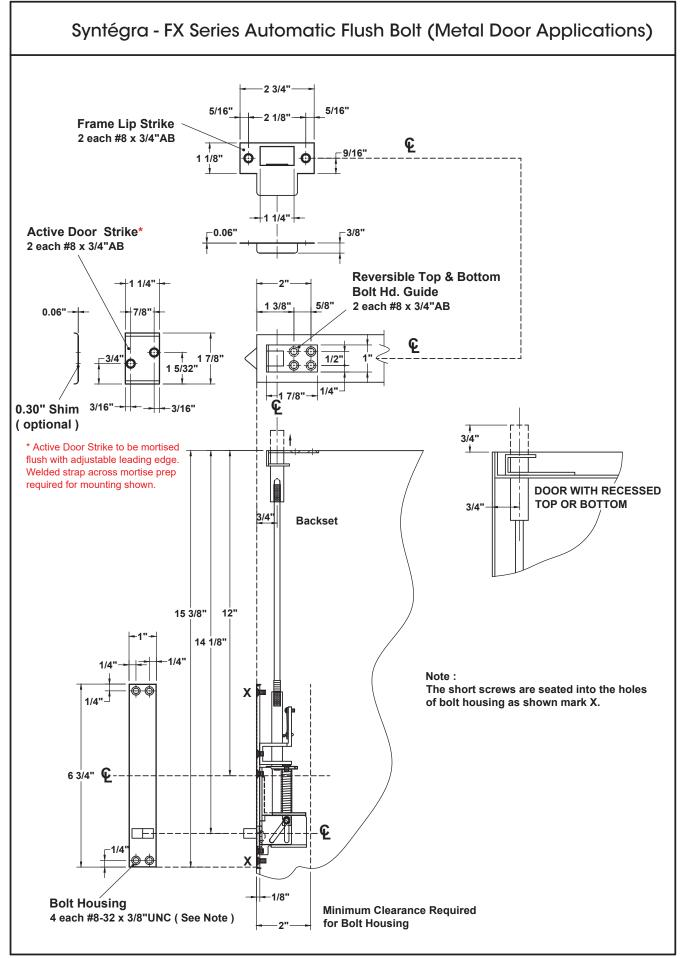
SCREW DETAILS: #8-32 x 3/8" UNC - flat countersunk head machine screw, total 4 pcs. #8 x 3/4"AB - undercut flat countersunk head, dual purpose machine/tapping screw, total 6 pcs.
